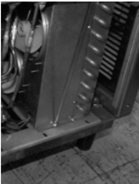
UNSCREW C-FAN MOTOR ASSEMBLY SECURING SCREWS LOCATED TOP AND BOTTOM FRONT SIDE, AND BACK SIDE
