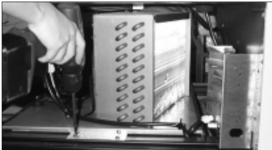
3. Unscrew four screws securing the Compressor Base.
