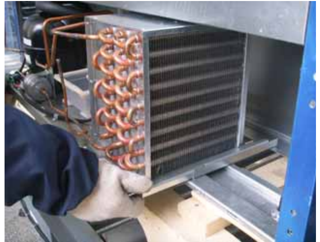
Pull out the condensing unit
