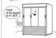
■ Set the front of the refrigerator a little bit higher than back-side by using adjustable feet to drain the water away with easily.
